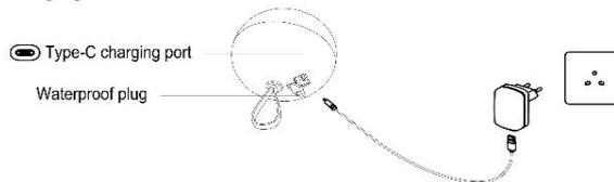
Open the waterproof plug and connect the USB cable to the Type-C port.
